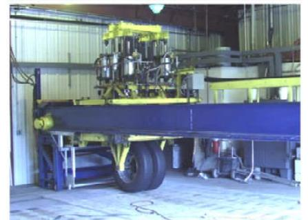
*Accelerated Pavement Testing facility*
