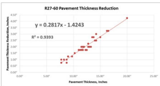
HMA pavement thickness reduction based upon former HMA thickness design.
