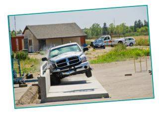
The group also evaluates the crash worthiness of proprietary hardware developed by others to ensure that it is acceptable for use on state highways. In addition, the group provides support to Caltrans Legal Division in tort liability cases by conducting crash tests and delivering technical assessments and expert witness testimony.
