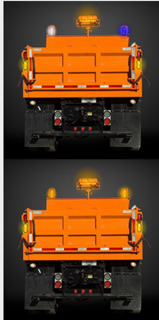
Visibility of snowplows is increased with blue and white lights (top) compared with traditional amber lights (bottom).
