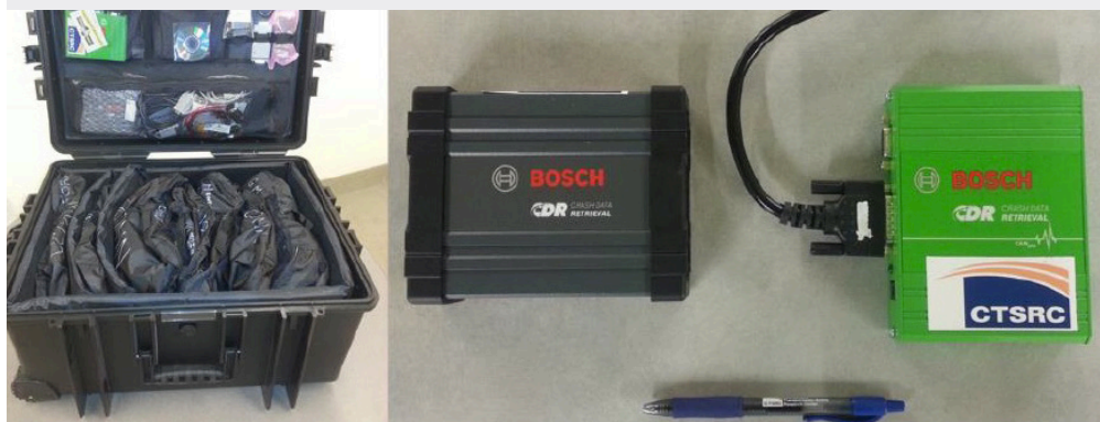
A download kit allows trained technicians to collect a vehicle's event data after a crash.
