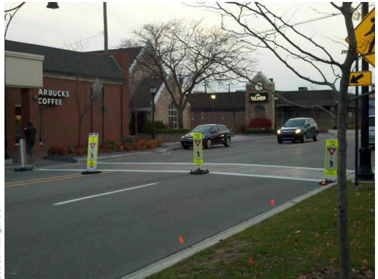
Four in-street signs comprise one version of the gateway pedestrian crossing configuration.
