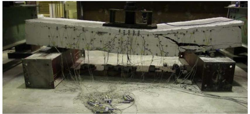
*Failure mode analysis in the lab showed that shear cracks did not penetrate to the UHPC layer but turned horizontally and began to separate the UHPC overlay section from the normal concrete base.*
