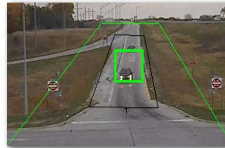
Emerging video analytics technologies have the potential to analyze video feeds from traffic cameras and detect crashes, congestion, stopped vehicles, wrong-way drivers, and other scenarios. If an incident is detected, the systems can create
