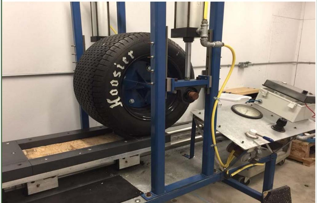
Automated trafficking machine used for simulating vehicle traffic in the laboratory
