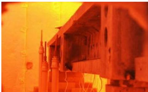
Concrete beams prestressed with CFRP strands were subjected to fire/loading tests to evaluate their fire endurance.
